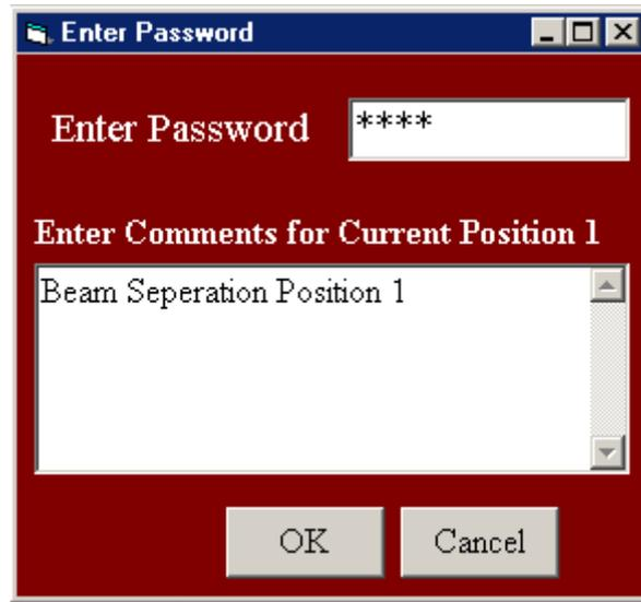
Once you set a position, a window appears with a message that indicates the movement of the motor. When the motor stops moving, the window disappears automatically.
