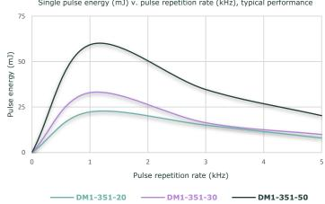
Single pulse energy (mJ) v. pulse repetition rate (kHz), typical performance
